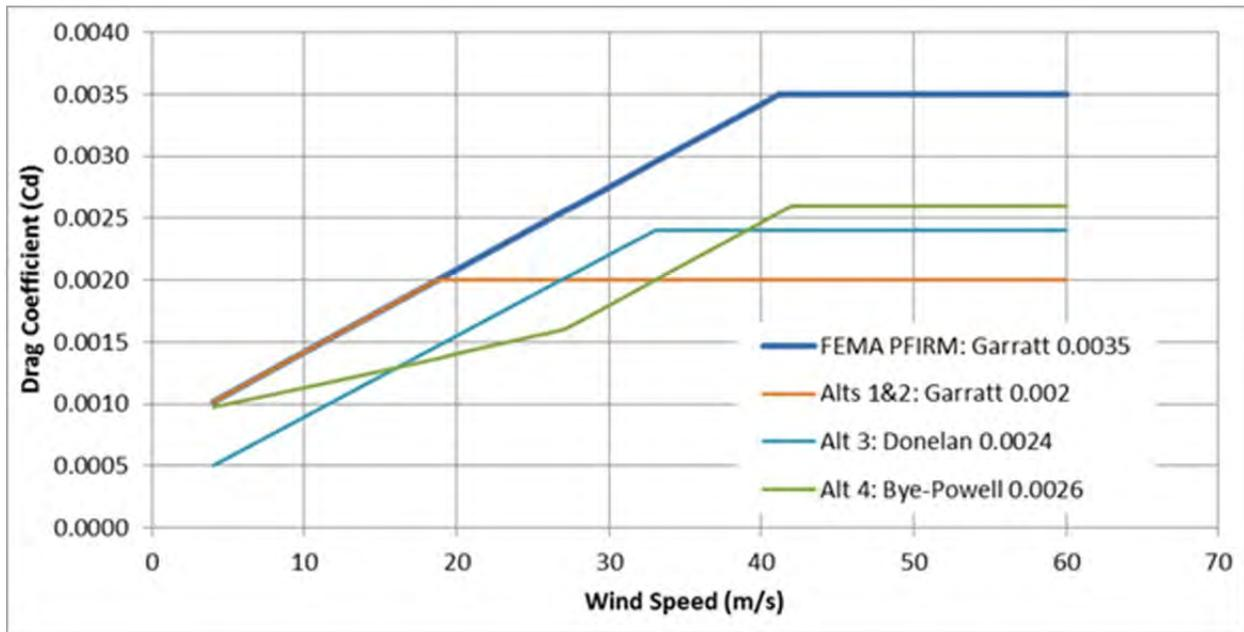
Figure 3-8. Alternative wind drag coefficient formulations tested.
